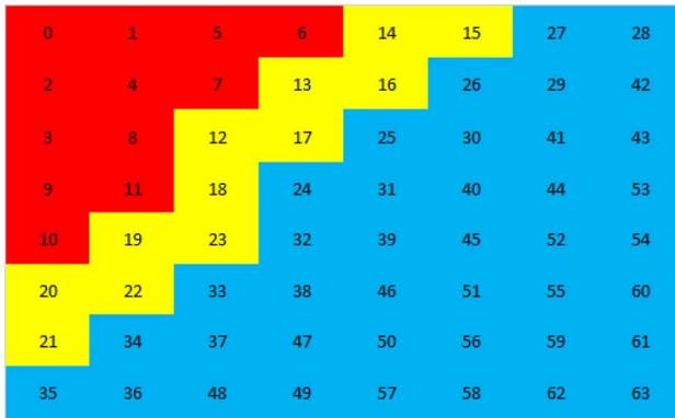
Fig. 2. Illustration of extension of splitting of transform coefficients into MGS layers without subdivision of an  $8 \times 8$  macroblock. For the example weights  $\mathbf{W} = [3, 3, 10]$ , the first  $4 \cdot w_1 = 4 \cdot 3$  coefficients form MGS layer 1, the next  $4 \cdot 3$  coefficients form MGS layer 2, and the remaining  $4 \cdot 10$  coefficients form MGS layer 3.
